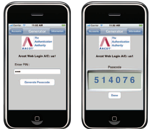
The user can use their mobile phone to automatically generate the one-time-passcode to be entered to gain access to their account or to complete the payment transaction
